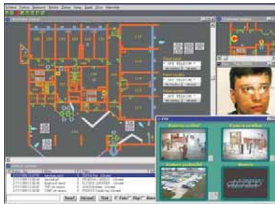
View of local installation screen in ALTEX with integrated ACS, ESS, EFS and CCTV modules.
