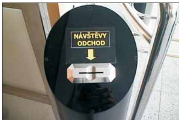
Access control solution with RDR-VIS-BOX card collector - detail.
